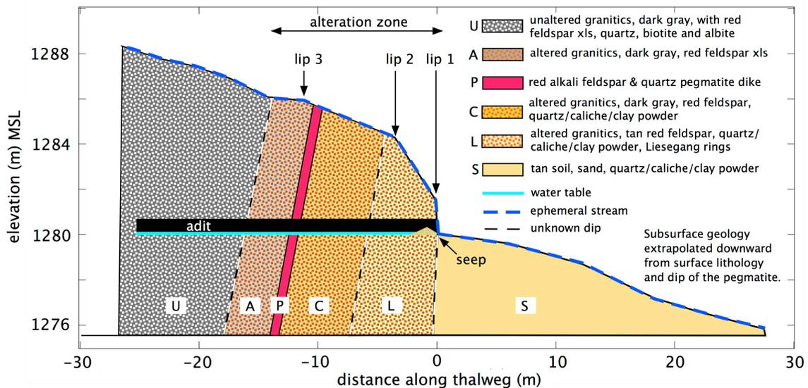
Figure 2. Surveyed elevation profile of the thalweg with rock units and water levels. Ivanpah Spring is indicated as the "seep". As judged by eye based on color, texture, gross mineralogy and the presence of yellow-orange powder, there were six different rock units (U, A, P, C, L and S). None of the subsurface dips are known, so the U-A, C-L and L-S contact dips are indicated with dashed lines. The A-P and P-C
